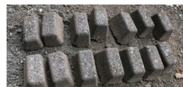
Water purification agents made from disposable body warmers
