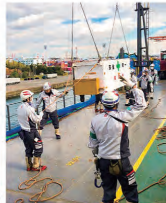
Training for using a crane to lift and transfer a lifesaving box from a vessel
